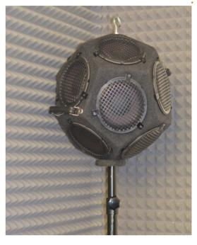
An omnidirectional sound source used in acoustic investigations
