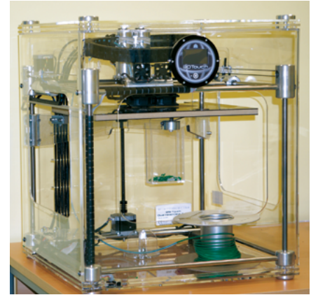
BFB 3D TOUCH Bits from Bytes 3D printer using FDM method
