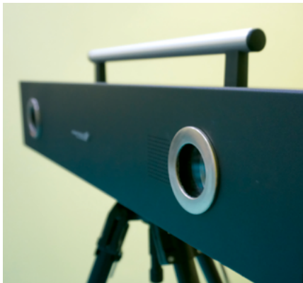
SCANBRIGHT PROFESSIONAL Smarttech – structural light 3D scanner
