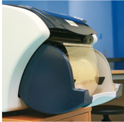
SOLIDO SD300 Solido 3D printer using LOM method
