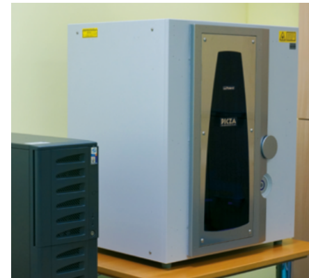
PICZA LPX-600 Roland – laser 3D scanner
